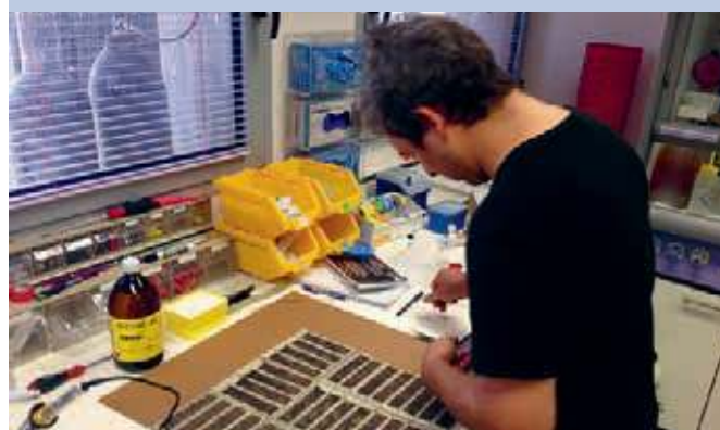
Fig. 3 - Lab testing of small scale SolarPaint coated units. SolarPaint develops a flexible net coated with its proprietary paint, that will produce electricity from the sun.
