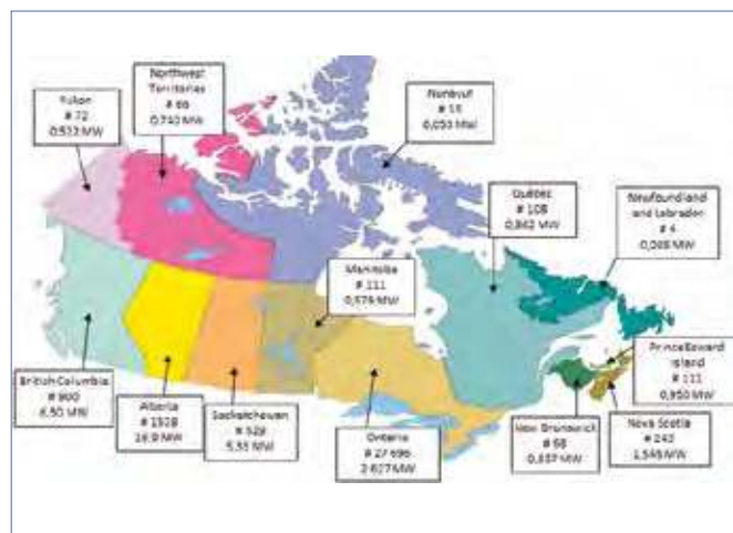
Fig. 1 - Map showing the Canadian provinces, the capacity (in megawatt), and the number of utility interconnected PV systems as of December 31 st , 2016. All power capacities are reported in DC (Watt peak, W p ).
