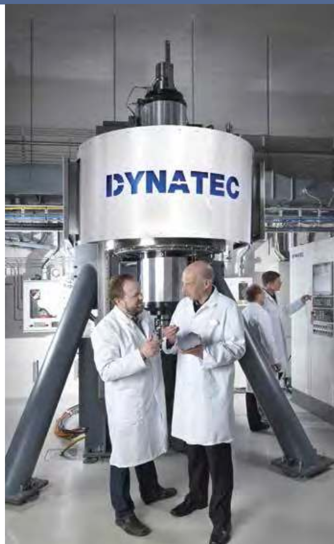
Fig. 1 - Efficient production of silicon feedstock is an important part of The Research Center for Sustainable Solar Cell Technology. Parts of this research are done with this prototype reactor for high rate pyrolysis of gaseous precursors (Photo: Jarle Nytingnes, Dynatec AS).
