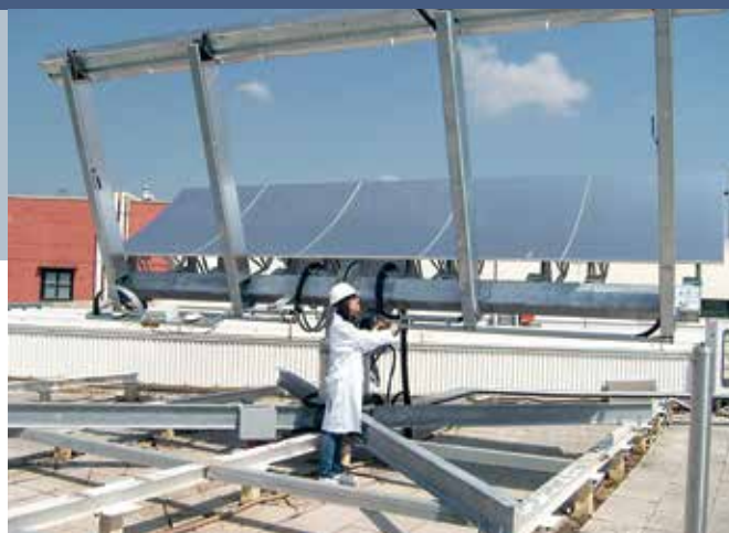
Fig. 2 – Hybrid concentrated PV-T, 2-axis tracking system (c.f. 60X – 1,7 kW E-power – 4,0 kW T-power) under test at ENEA Portici Research Centre.
