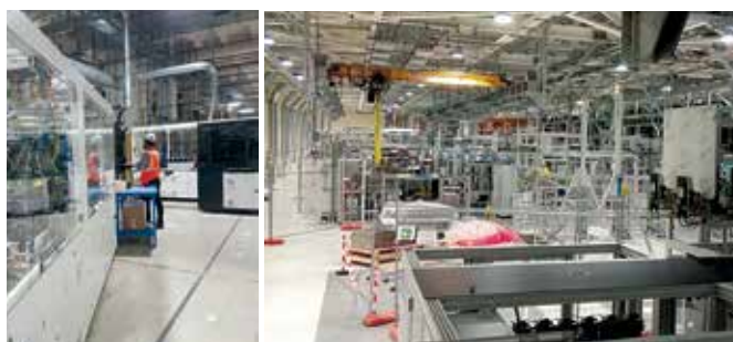
Fig. 3 – EGP PV module factory: Cell stringing phase of module assembly line (started on Jul 2018) and HJT cell lines (will be completed on June 2019).
