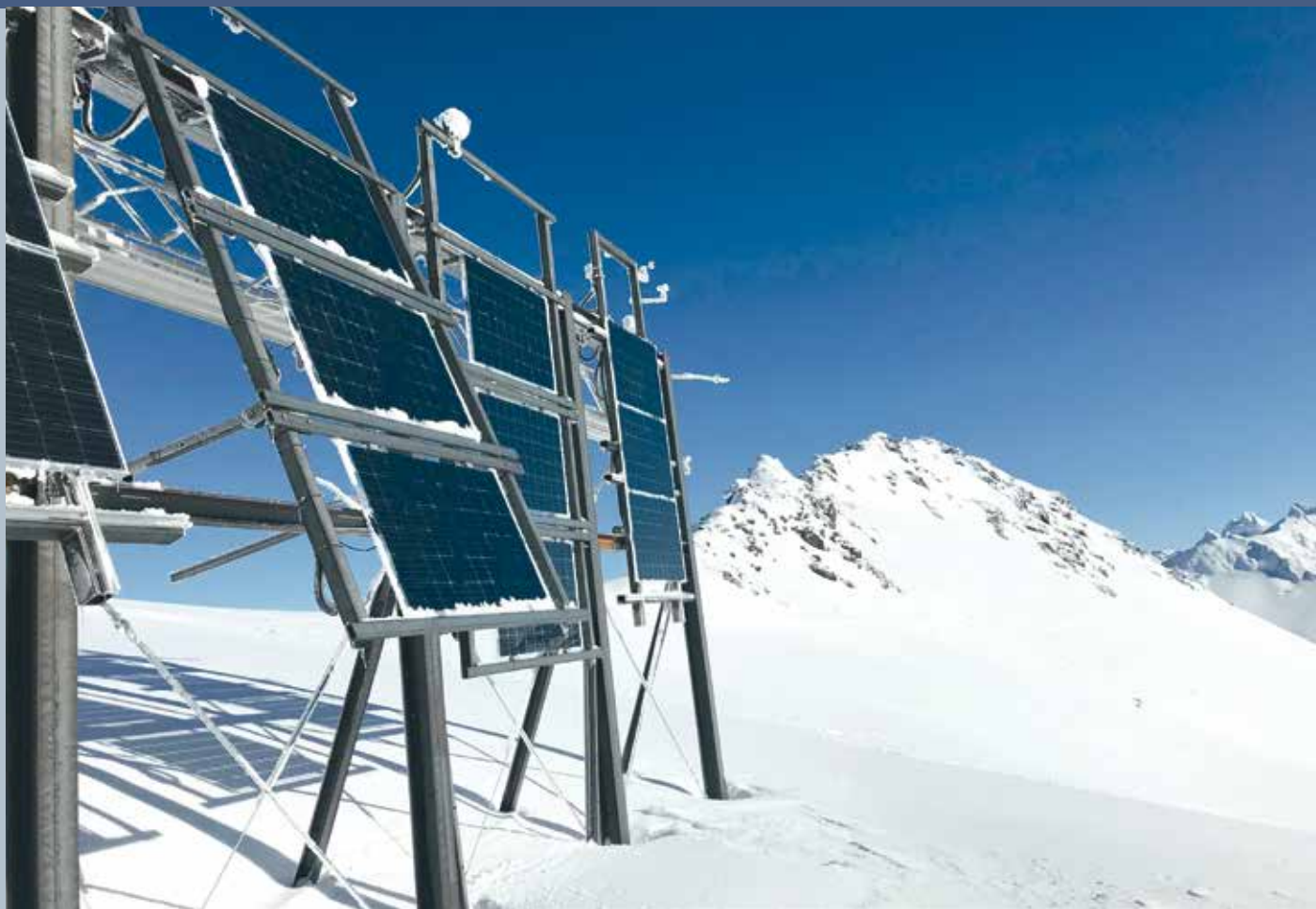
Fig. 1 – Installing photovoltaic panels in high mountains could reduce the power deficit experienced in winter, according to a recent study by the WSL Institute for Snow and Avalanche Research SLF and EPFL (Annelen Kahl, Jérôme Dujardin, and Michael Lehning, PNAS January 22, 2019 116 (4) 1162-1167) (Photo: © ZHAW Wädenswil).
