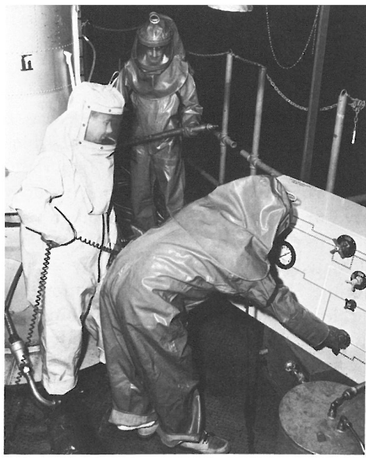
Martin Co. and Aerojet General Corp. personnel wear protective clothing while fueling the Vanguard second stage with white inhibited fuming nitric acid.
