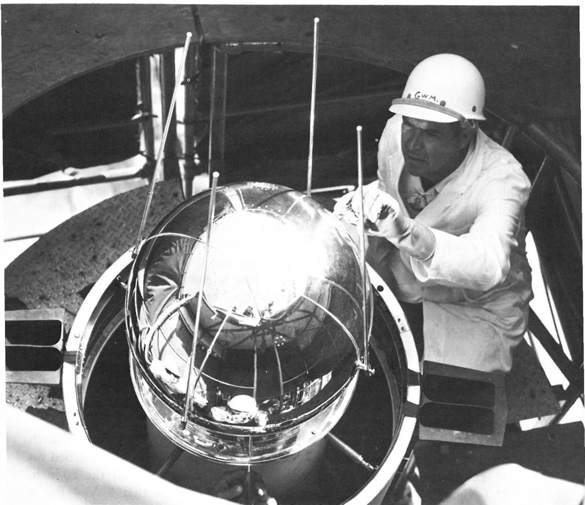
Sketch and photograph of the first of the “operational” twenty-inch Vanguard satellites. It was launched by TV-5, 28 April 1958, but failed to achieve orbit because the third stage did not fire.
