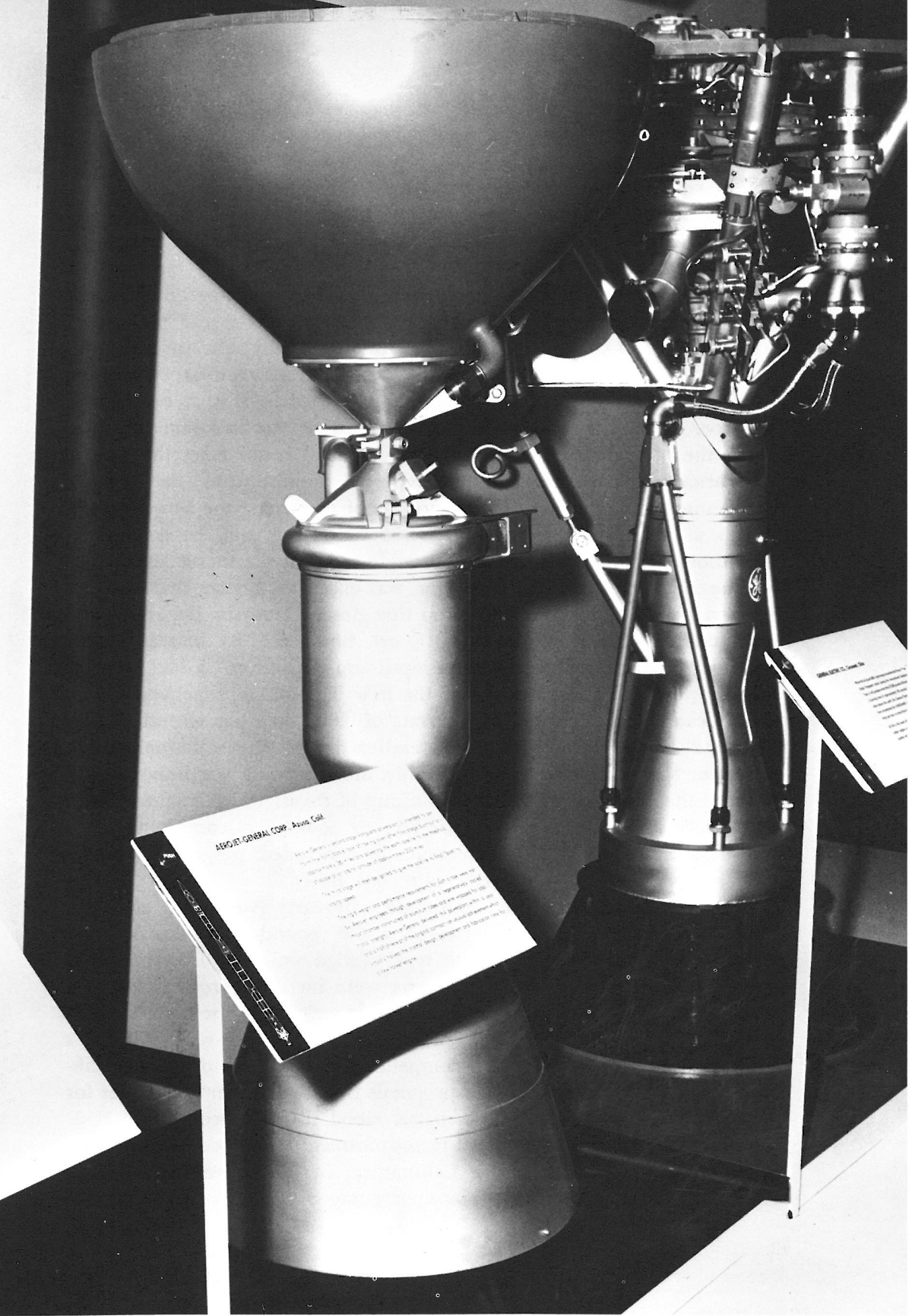
Vanguard engines: rear, GE's first-stage engine; foreground, Aerojet General's second-stage engine.
