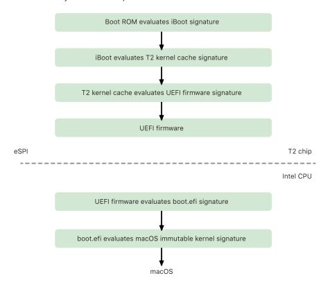
After verification, the UEFI firmware image is mapped into a portion of the T2 chip memory. This memory is made available to the Intel CPU through the enhanced Serial Peripheral Interface (eSPI). When the Intel CPU first boots, it fetches the UEFI firmware through the eSPI from the integrity-checked, memory-mapped copy of the firmware located on the T2 chip.
