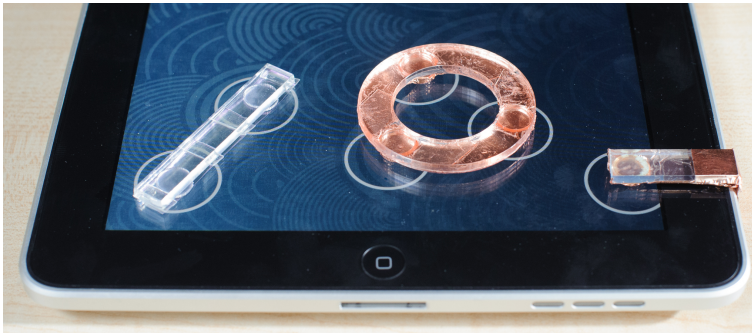
Figure 2.2: Passive Untouched Capacitive Widgets (PUCs). They are uniquely identified through the pattern of the contact points. [Voelker et al., 2013]
