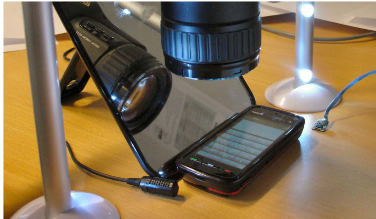
Figure 2.4: Hardware to measure latency by Kaaresoja and Brewster [2010]. A touch display is placed on the table along with a mirror beside it. A camera is mounted to capture a slow-motion video with both the mirror and the touch display in the frame.
