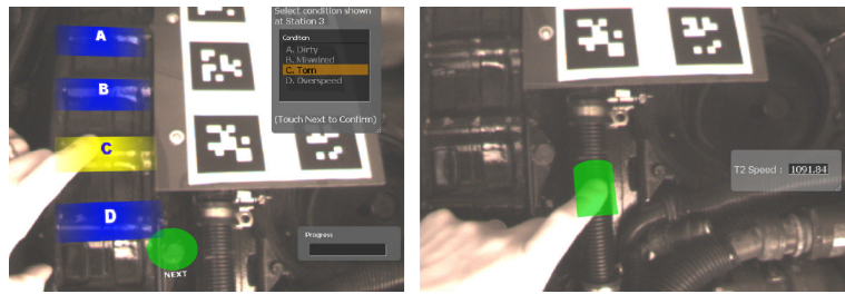
Figure 3.1: Opportunistic Controls [Henderson and Feiner, 2008]: Example for virtual controls aligned with physical characteristics. Left: virtual buttons on raised parts of an engine housing. Right: virtual slider on a wiring harness with grooves.
