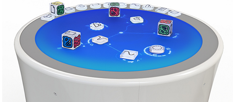
Figure 1.1: The Reactable is a prominent example of a TUI. Music can be played and changed by physical objects placed on the surface.
