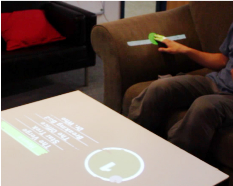
Figure 3.3: WorldKit [Xiao et al., 2013]: Virtual Controls can be placed on any surface and interact with each other. Here, a digital TV guide and a volume control are displayed on the table as well as a virtual slider to dim the light on the arm rest of the couch.
