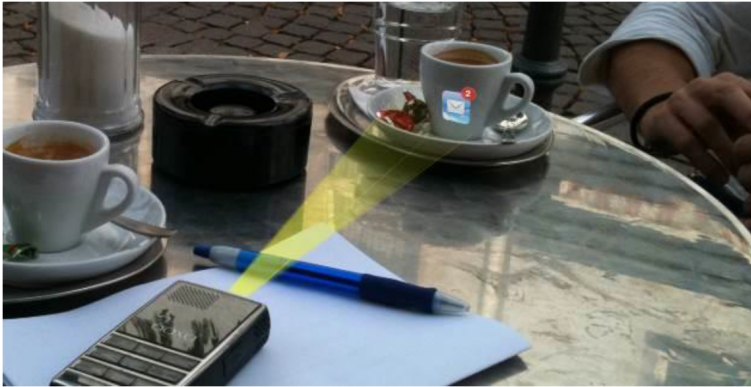
Figure 3.4: LightBeam [Huber et al., 2012]: A pico projector and a depth camera turn objects into interactive displays that react to touch input.
