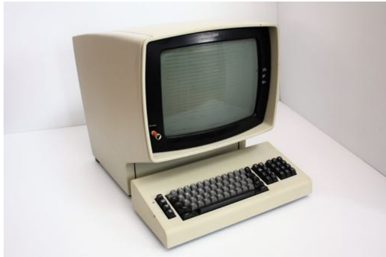
Figure 2.2: The IBM 3277 CRT was able to display 40 \times 24 characters in green color on a dark background. Image adapted from https://vintagecomputer.ca .
