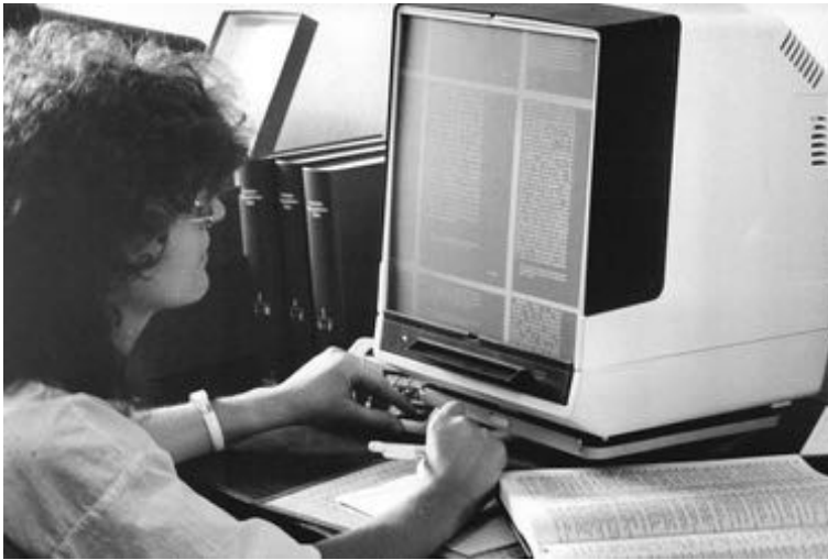
Figure 2.3: A microfiche reader. The flat microfiche film contains multiple images with a size of about 10 \times 14 \text{mm}^2 each. The device magnifies these small images and displays them on the screen. Image adapted from https://commons.wikimedia.org .
