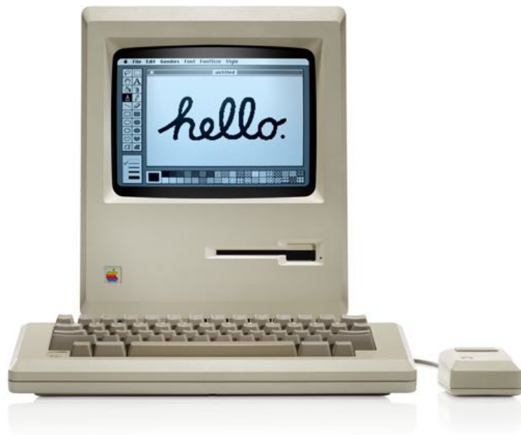
Figure 2.1: The Apple Macintosh 128k was released in 1984 and had a resolution of 512 \times 342 pixels. Image adapted from http://blog.archive.org .
