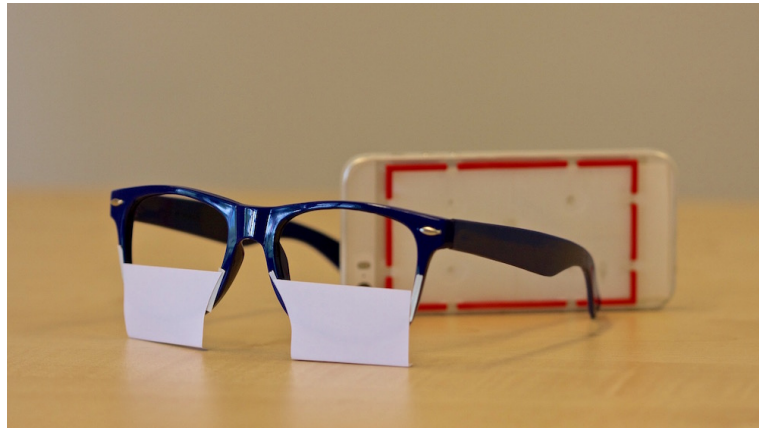
Figure 5.2: The blocker glasses we used in the study and a phone equipped with tactile landmarks in the background
