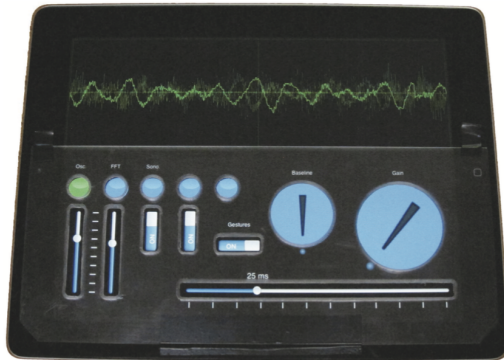
Figure 2.2: iPad equipped with tactile overlays used in the study by Kincaid. Taken from: "Tactile Guides for Touch Screen Controls" by Kincaid [2012]
