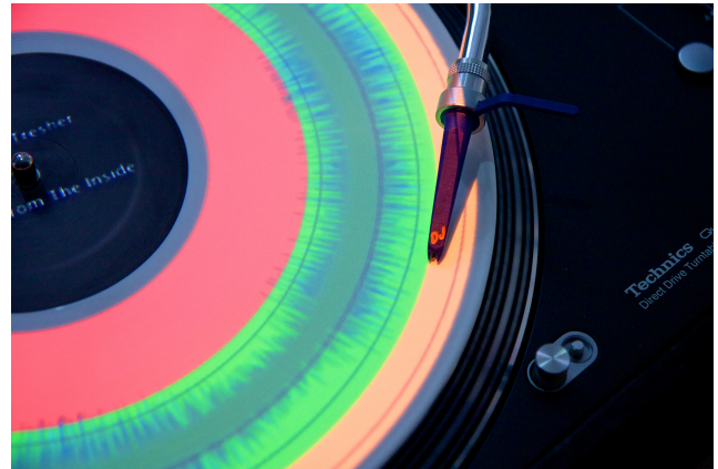
Figure 1: DiskPlay visualizes track length, playback progress, cue points and the waveform on a timecode vinyl.
