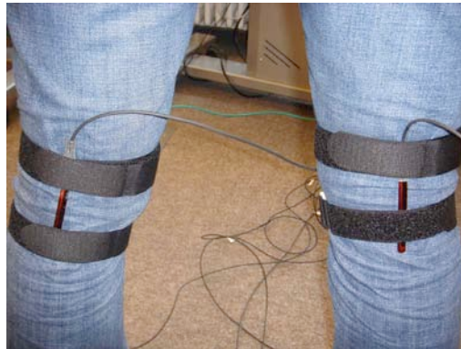
Figure 5.2: Bend sensors attached to the back of the knee via velcro straps.
