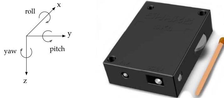
Figure 2.7: SHAKE SK6 IMU and its axes. It calculates orientation with respect to a fixed coordinate system.
