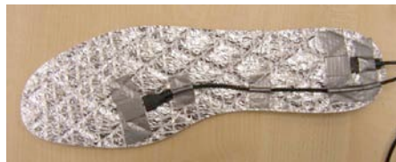
Figure 5.1: Two FSRs taped on the bottom side of a shoe insole.
