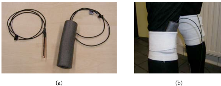
Figure 6.6: (a) The right bend sensor is protected by a thick foam. (b) Bend sensors attached with knee pads.
