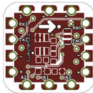
Figure 3.18: LumiNet 2 V2.0 board design, top side.
