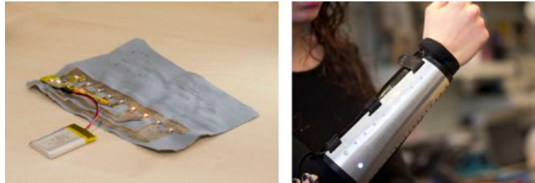
Figure 3.11: Hand guard design with LumiNet 2 prototype
