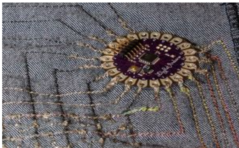
Figure A.3: Skirt display back side detail.
