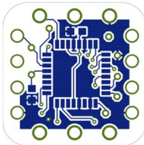
Figure B.2: LumiNet 2 v2.0 hardware board bottom layer.
