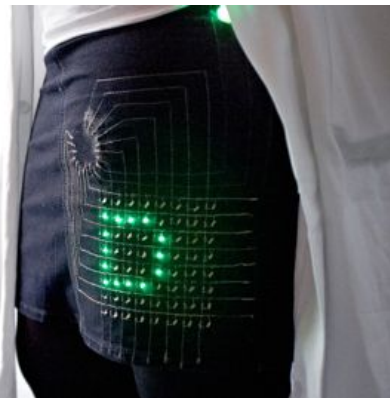
Figure 3.3: The skirt with LED matrix controlled by a LilyPad.
