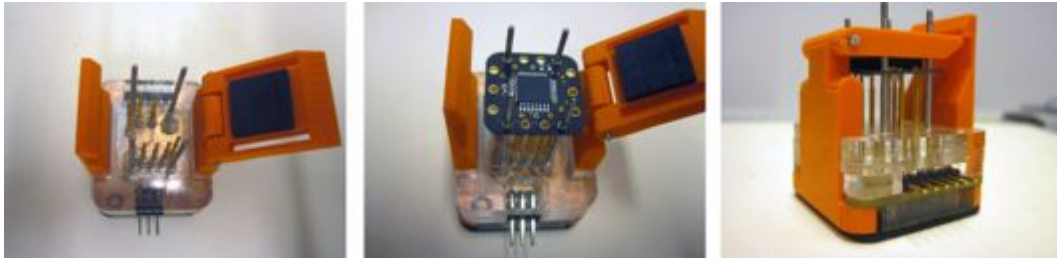
Figure 3.16: LumiNet 2 pogo pin adapter.
