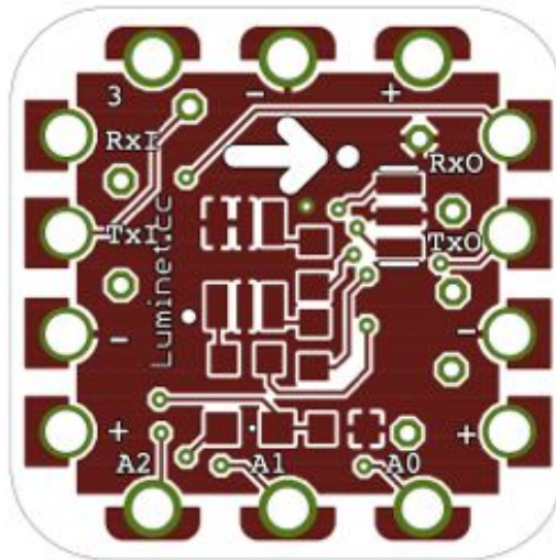
Figure B.1: LumiNet 2 v2.0 hardware board top layer.
