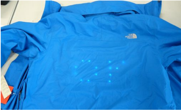
Figure 4.5: Luminet2 node controlling an 8 by 8 matrix of LED made with addressable flexible LED strips.
