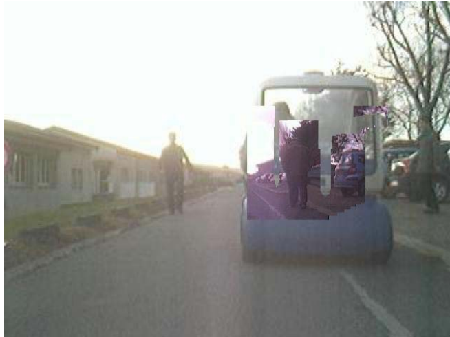
Fig.15. Cooperative augmented reality (CAR): 'see' through the occlusion
