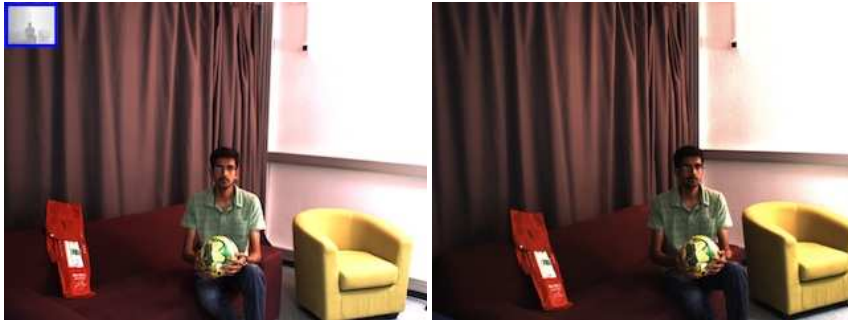
(b) A high-resolution color image pair with the low-resolution ToF image shown in the upper-left corner of the left image at the true scale.
