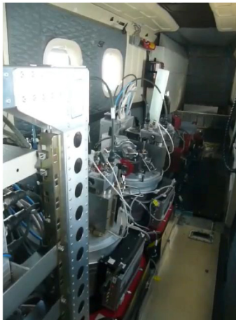
Fig. 4. Sieleters filmed during in-flight data acquisition. The two platforms in red in Media 2 seem to be mechanically welded, while they are totally independent, in terms of hardware and software.
