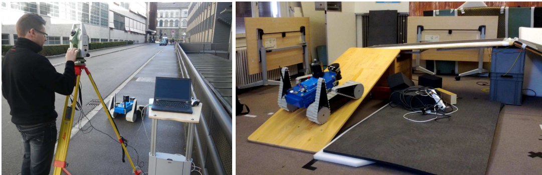
Figure 5: The experimental setup with the Leica reference theodolite for obtaining ground truth trajectory (left). Part of the 3D semi-structured environment for indoor test with motion capture ground truth (right).
