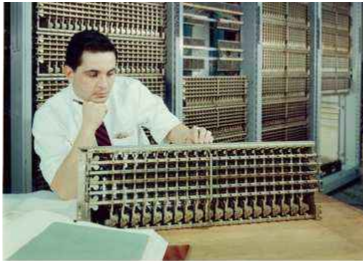
Fig. 5-15. The crossbar switch was developed at Bell Labs and first installed in the Bell System in 1938 and saw service until the early 1990s. The basic switch was a 10-by-20-matrix switch, consisting of electromechanical relay contacts. [1960 photo courtesy of Alcatel-Lucent USA Inc. / Bell Labs.]
