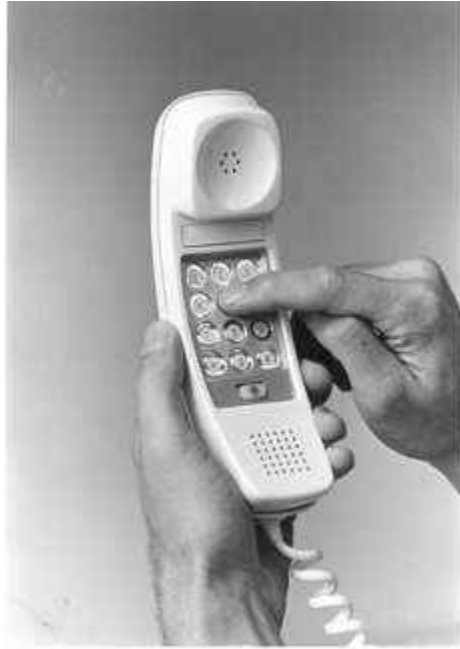
Fig. 5-17. Touchtone dialing, with push-button dials, replaced rotary dial in telephone instruments, starting in 1963. Today few people would have encountered a rotary dial. Shown here is a Trimline® telephone with the Touchtone dialer in the handset. [Photo courtesy of Alcatel-Lucent USA Inc. / Bell Labs.]
