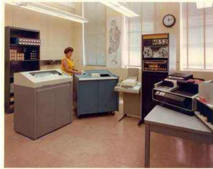
Fig. 3-2. Punched cards were used for batch processing on computer systems in the 1960s and even the 1970s. Here in 1973 cards are being read in a card reader. [Photo courtesy of Alcatel-Lucent USA Inc. / Bell Labs.]
