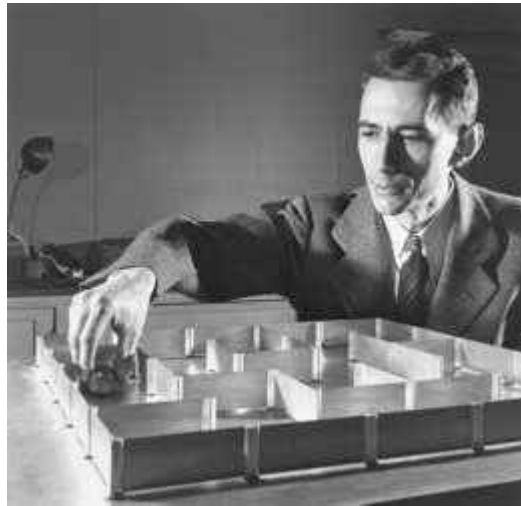
Fig. 5-9. Claude E. Shannon in 1952 with his electrically controlled mechanical mouse, named “Theseus.” The mouse, through trial and error, would “learn” the solution to the maze through electromechanical relays and was an example of “intelligent behavior.” [Photo courtesy of AT&T Archives and History Center.]
