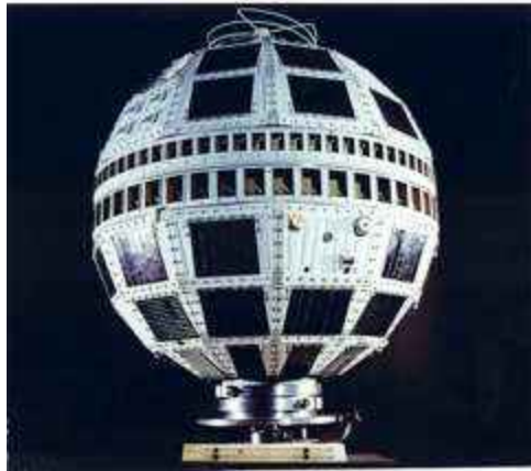
Fig. 5-13. The active communications satellite Telstar was placed in low-Earth orbit in 1962 and relayed telephone, television, and facsimile signals. This heralded the beginning of satellite telecommunications. [Photo courtesy of Alcatel-Lucent USA Inc. / Bell Labs.]
