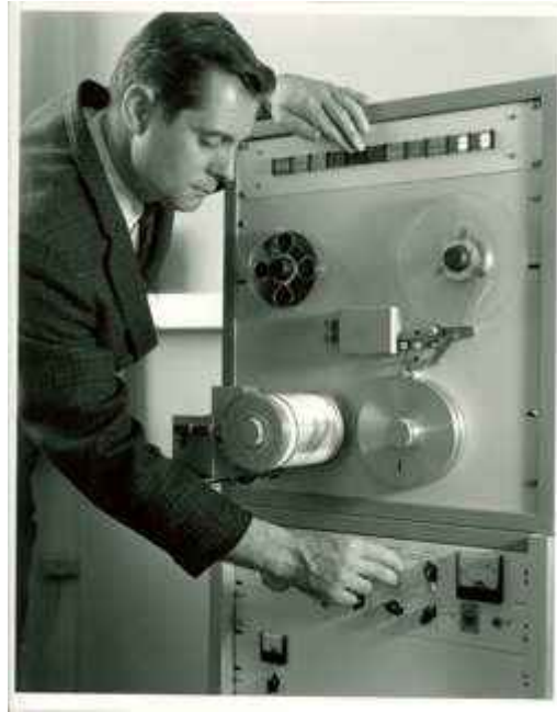
Fig. 5-18. The sound spectrograph machine made a two-dimensional analysis of the frequency components in a sound signal and displayed the results on a rotating drum. In this photograph from 1966, Toni Presti is shown adjusting the spectrograph machine. Today such sound spectrographs are made in real time with software in hand-held tablet computers. The spectrograph was important in secure speech processing and in underwater sound. [Photo courtesy of Alcatel-Lucent USA Inc. / Bell Labs.]
