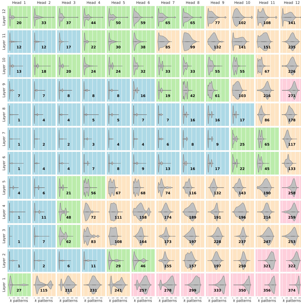
Figure A.3: Analysis of operating modes of the heads of a pre-trained BERT model. For each head in each layer, the distribution of the minimal number k of patterns required to sum up the softmax values to 0.90 is displayed as a violin plot in a panel. k indicates the size of a metastable state. The bold number in the center of each panel gives the median \bar{k} of the distribution. The heads in each layer are sorted according to \bar{k} . Attention heads belong to the class they mainly operate in. Class (IV) in blue: Small metastable state or fixed point close to a single pattern, which is abundant in the middle layers (6, 7, and 8). Class (II) in orange: Large metastable state, which is prominent in middle layers (3, 4, and 5). Class (I) in red: Very large metastable state or global fixed point, which is predominant in the first layer. These heads can potentially be replaced by averaging operations. Class (III) in green: Medium metastable state, which is frequently observed in higher layers. We hypothesize that these heads are used to collect information required to perform the respective task. These heads should be the main target to improve transformer and BERT models.
