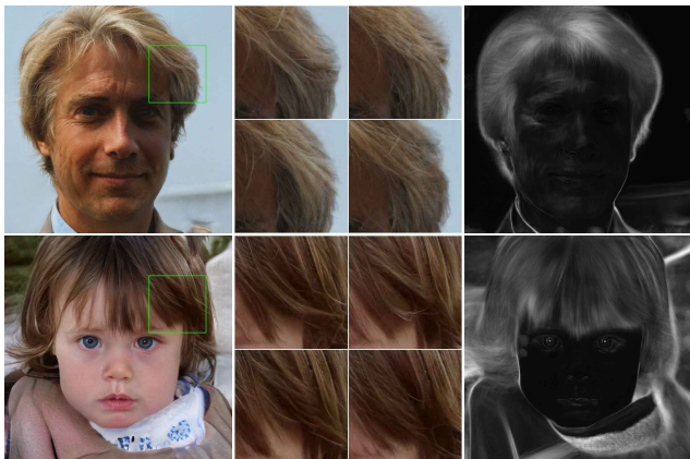
Figure 4. Examples of stochastic variation. (a) Two generated images. (b) Zoom-in with different realizations of input noise. While the overall appearance is almost identical, individual hairs are placed very differently. (c) Standard deviation of each pixel over 100 different realizations, highlighting which parts of the images are affected by the noise. The main areas are the hair, silhouettes, and parts of background, but there is also interesting stochastic variation in the eye reflections. Global aspects such as identity and pose are unaffected by stochastic variation.
