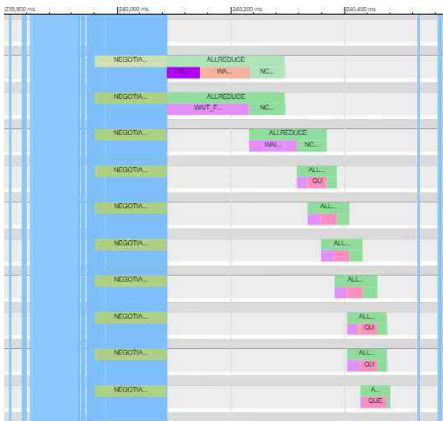
Figure 2. Horovod Timeline to illustrate the improved orchestration with grouping and bitvector allreduce. The blue vertical lines are cycle markers.
