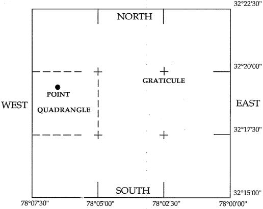
Point: Latitude 32°18'48" North, Longitude 78°06'05" West Note: This diagram is based on a USGS 7.5 Minute Series Topographic Map. It is not drawn to scale.
