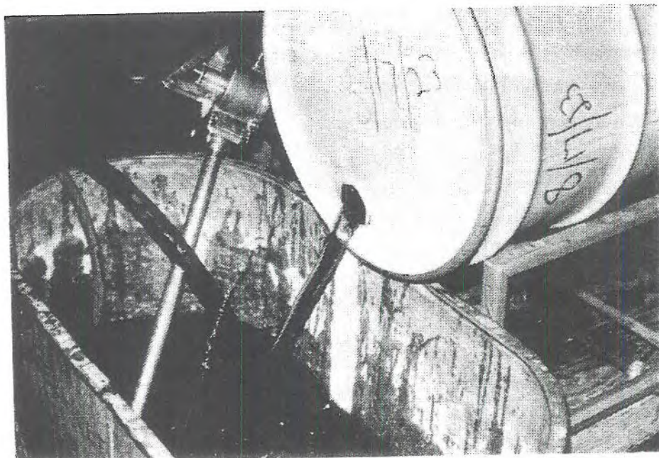
Figure A-4. 55-Gallon, (0.21m 3 ), steel, open-top drum (lid attached) resting on drum dolly while pouring motor oil into trough.
