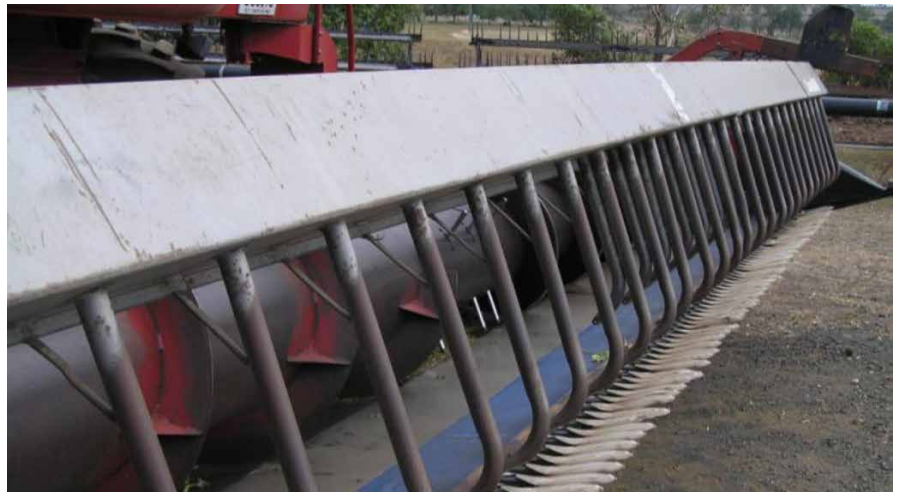
Photo 2: Harvestaire front combined with extension fingers and a blue vibra-mat.
