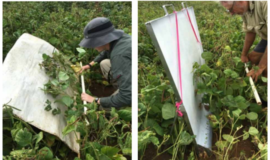
Photo 81: The traditional soft cloth beat sheet (left) and a rigid aluminium beat sheet (right) with collecting trough at the base, as used in 0.25 m rows of mungbeans.
