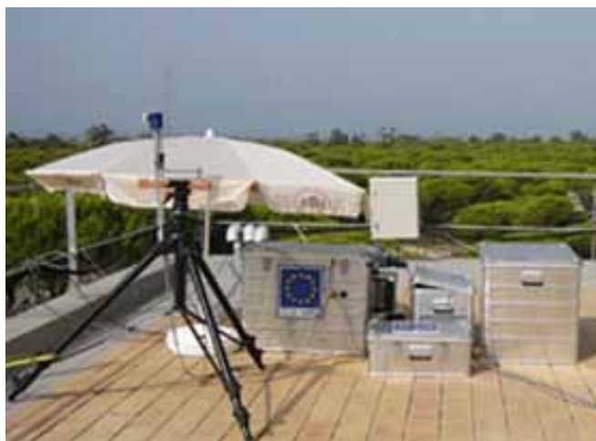
Figure 21: The traveling spectroradiometer QASUME installed at El Arenosillo, Spain [59].
