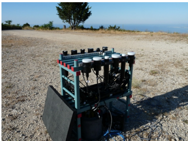
Figure 20: The intercalibration bench used in the frame of the BOUSSOLE project [55].
