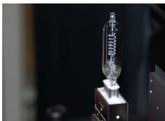
Figure 3: An FEL lamp will be used as a stable irradiance source for indoor intercomparison.
