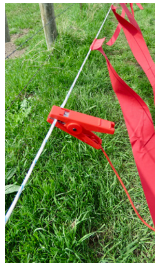
Some energizers come with alligator clamps on insulated wire that are useful for making strong hot and ground wire connections.
