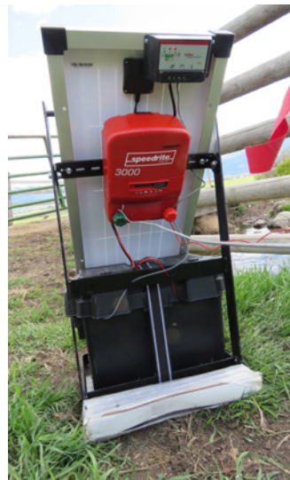
The front and back of a solar energizer with a red wire leading from the hot terminal (the red knob) to the fladry poly wire and a steel wire leading from the ground terminal (the green knob) to the ground rods.
