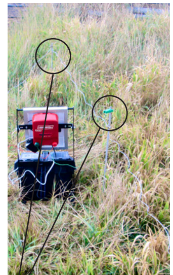
The ground rods on the right side of this image are connected to each other using wire and metal clamps and are connected to the energizer using a green alligator clamp.
