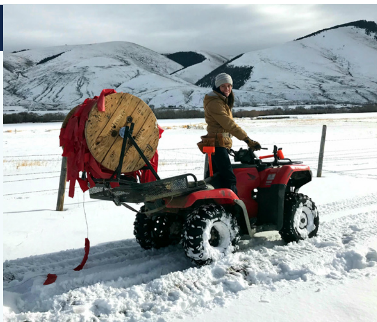
A fladry spooler connected to the back of an ATV or truck is the most efficient way to spool out fladry and can also be useful for respooling the fladry line when taking the fladry fence down.
