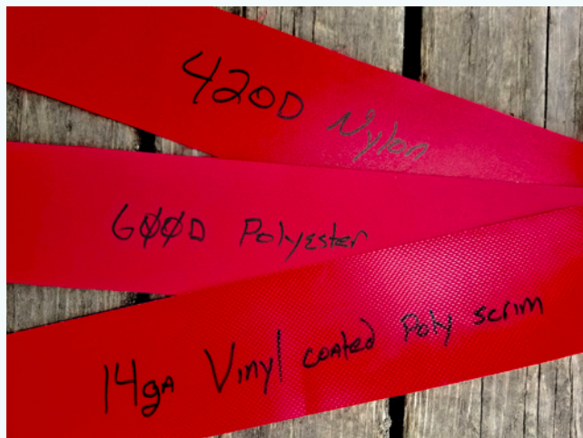
The three types of fladry materials sold by Jonco Industries have different weights and textures.
