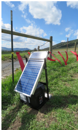
The front and back of a solar energizer with a red wire leading from the hot terminal (the red knob) to the fladry poly wire and a steel wire leading from the ground terminal (the green knob) to the ground rods.
