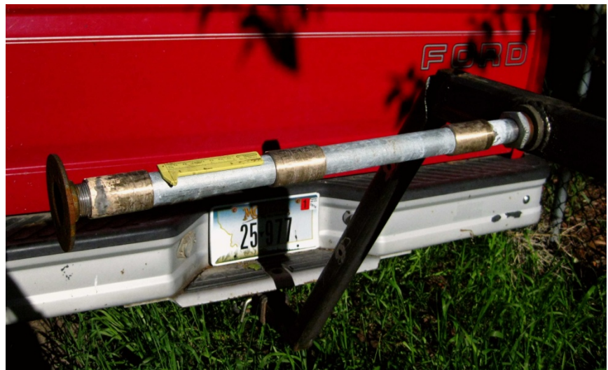
Figure F: 1" nominal pipe spindle, with bronze bushings for smooth spool rotation. Three bushings to accommodate different size spools.
