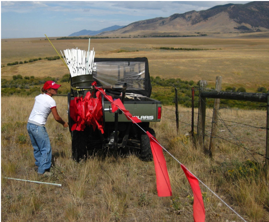
Figure A: Spooler 2.0, which included a level-winding device to evenly distribute the fladry on the spool. The level winder has been omitted from subsequent designs.
