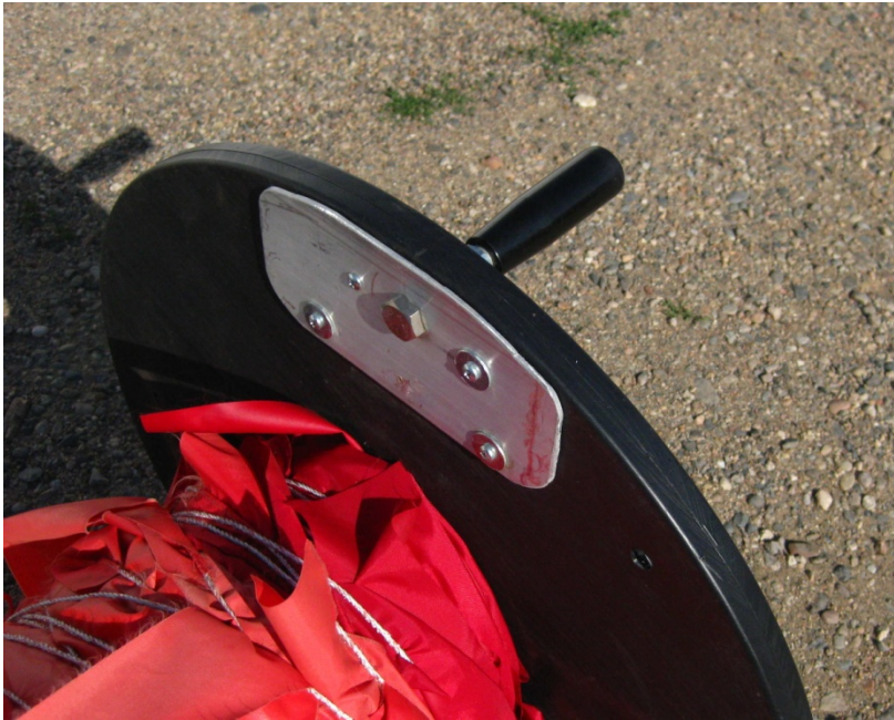
Figure G: Removable spool handle attached to flange.
