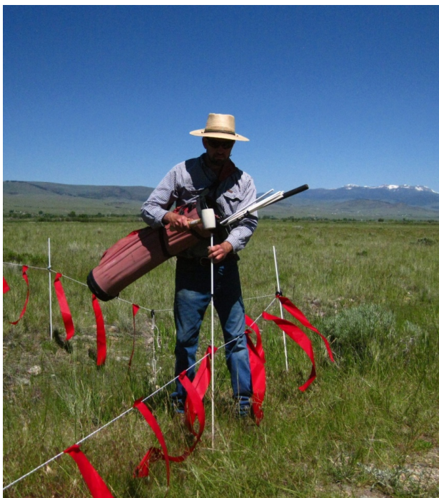
Figure 5: Using a golf bag for posts leaves hands free for positioning and hammering posts.
