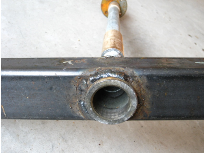
Figure C: Pipe coupling detail; coupling can be accessed from either side of frame for versatility.
