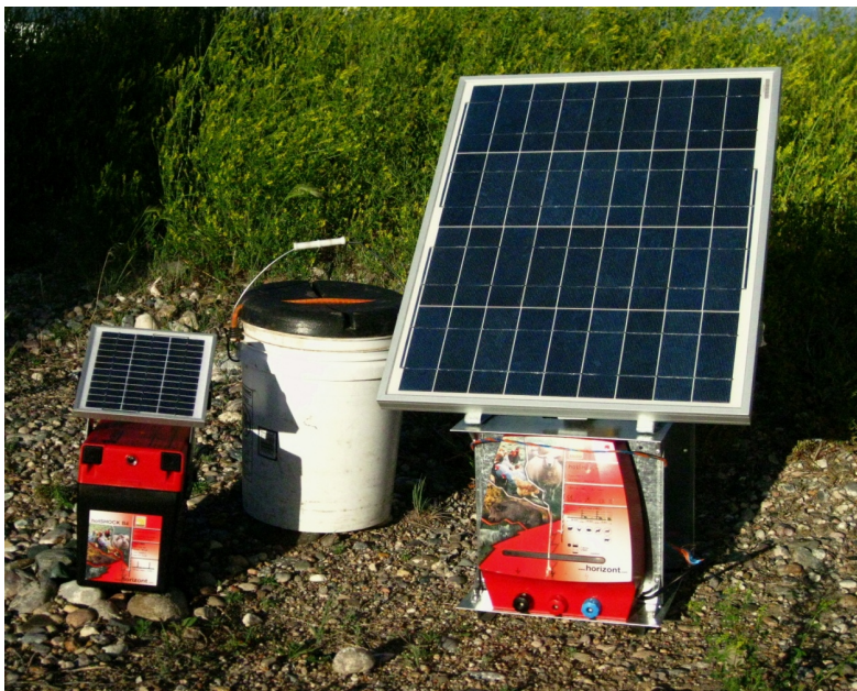
Figure 15: Horizon wide-impedance energizers with solar panels. The Hotshock B4 (left), with 0.35 output joules, is a compact unit that is suited for smaller runs of fladry around corrals or small pastures. The Hotshock A50 (right) is a heavy-duty unit that can adequately power more than 3 miles of electrified fladry; its 40-watt solar panel ensures a well-charged battery.
