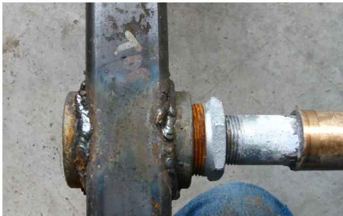
Figure D: Top view of pipe coupling welded into 3x2 tube; note reducing bushing on right receiving 1" pipe as spindle.
