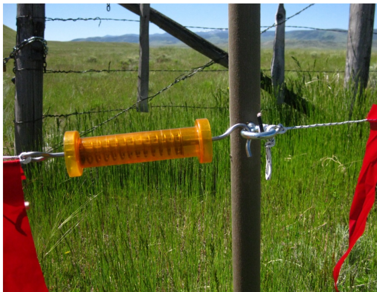
Figure 13: Gate handle connected to eye-bolt, attached to a Powerflex composite post.
