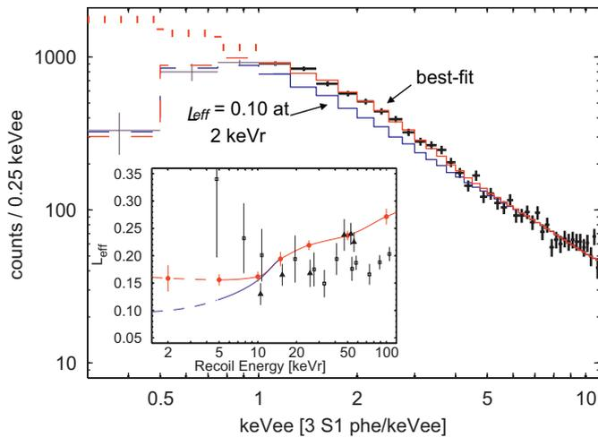
**Fig. 7.** A scenario in which  $\mathcal{L}_{\text{eff}}$  continues to fall below 10 keVr, to 0.10 at 2 keVr (as shown inset, blue line) is inconsistent with our data. The best-fit Monte Carlo (red line) and energy dependence of  $\mathcal{L}_{\text{eff}}$  (inset, red line) are as shown in Figs. 2 and 3. For interpretation of the references to color in this figure legend, the reader is referred to web version of this article.
