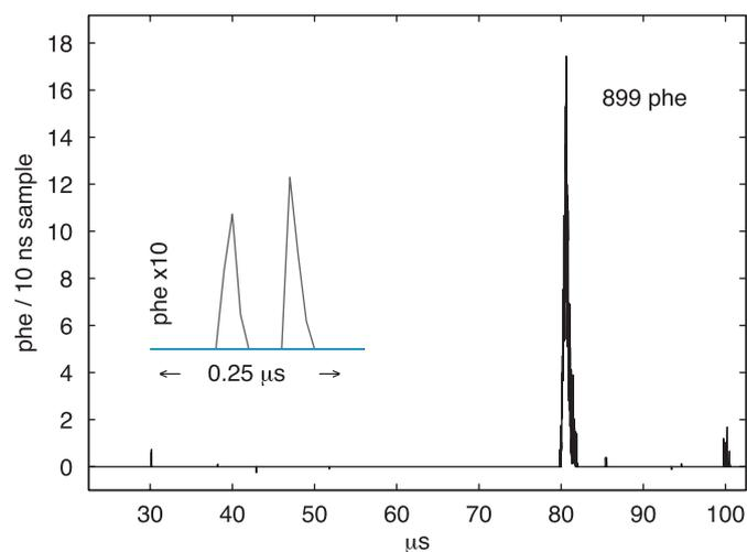
**Fig. 6.** An elastic nuclear recoil event at 0.75 keVee. The  $S_1$  signal of 2.3 photo-electrons at  $30 \mu\text{s}$  is also shown inset  $\times 10$  in  $y$  and  $\times 100$  in  $x$ . The  $S_2$  signal consists of 899 photo-electrons (about 37 ionization electrons). The small pulse at  $100 \mu\text{s}$  is a 22 photo-electron  $S_2$  from a single ionization electron. Baseline fluctuations of up to  $0.10 \pm 0.03$  photo-electrons/sample were set to zero in the analysis.
