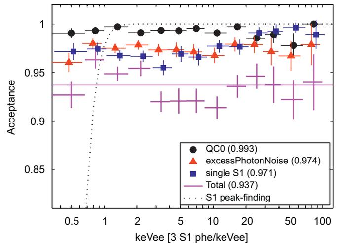
**Fig. 5.** Event acceptance for single-scatter nuclear recoils in the fiducial target. Average acceptance 0.5–100 keVee is indicated in the legend. The cuts are described in Section 3.2. The S1 peak-finding efficiency is discussed in Section 3.3.
