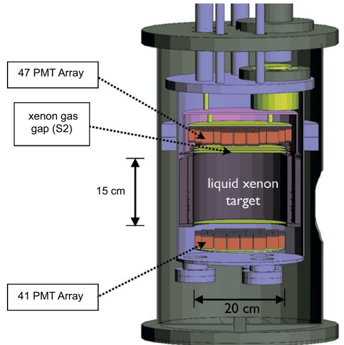
**Fig. 1.** A side view cut-away schematic of the XENON10 detector as rendered by the GEANT4 simulation. The liquid xenon target is 15 cm in height with a 20 cm diameter. Ancillary systems, cabling, shielding, etc. are omitted for clarity. The detector was completely enclosed by 20 cm Pb outside of 20 cm polyethylene shielding.
