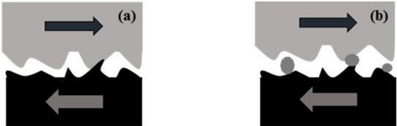
Figure 2: Schematic of (a) two-body and (b) three-body abrasive wear.
