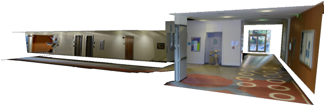
Figure 7: 3-D textured rendering of one of the walls of the reconstructed Corridor 2 scene.
