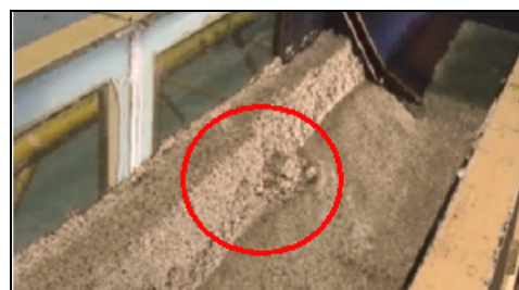
Figure 6b Bank erosion resulting from intermittent block failure
