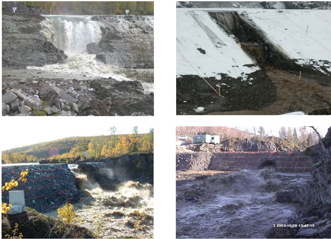
Figure 1 Breach development stages (4 different field tests)
