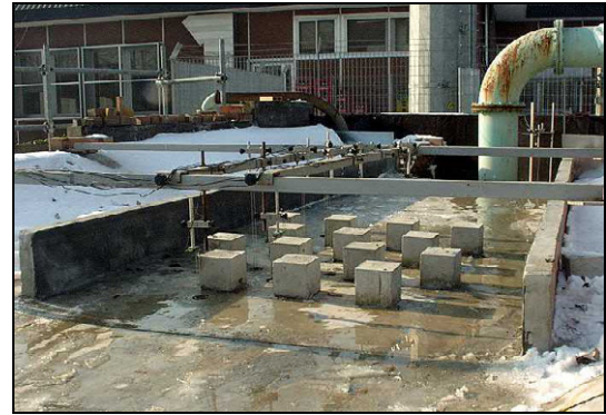
Figure 4b Physical modelling of flow through a mesh of buildings
