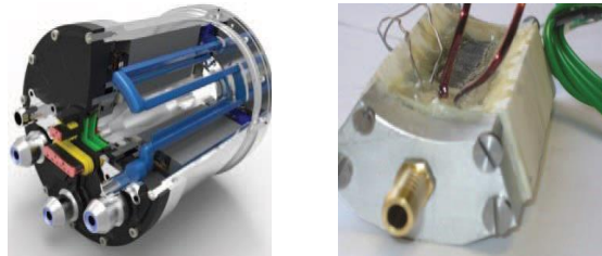
Fig. 16. Slot duct cooling for the whole motor (left) and single teeth prototype (right) [55].
