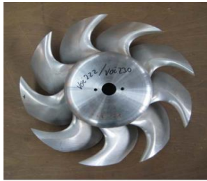
Fig. 5. The axial fan with forward swept and inclined blades [39].
