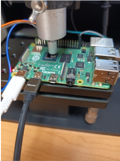
Figure 4: Raspberry Pi board with EM probe positioned on the ARM Cortex A72 Processor
