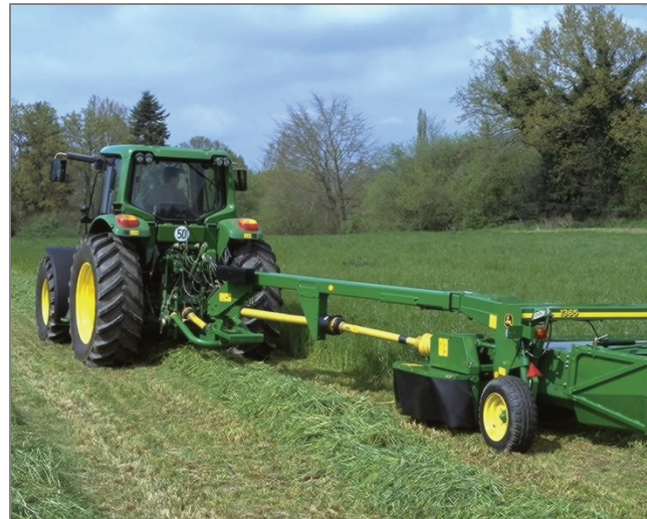
Figure 4. PTO driveline on mower conditioner, showing shields.
