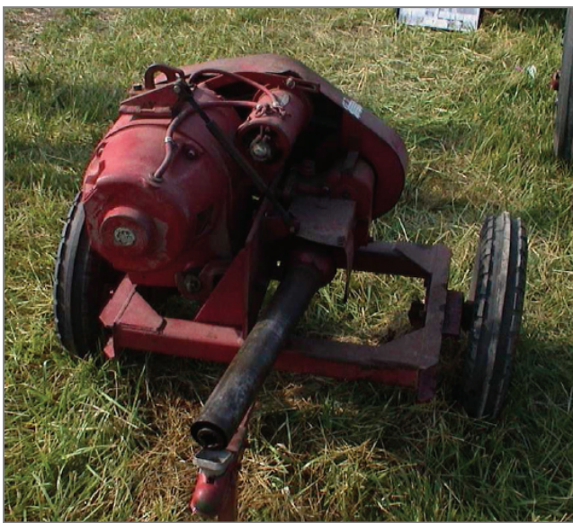
Figure 24. PTO-driven generator, retrofit power generation device.
