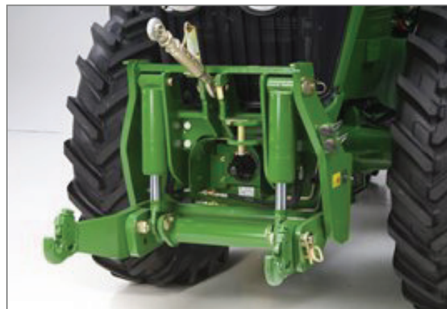
Figure 5. Typical bolt-on front PTO and three-point hitch module.
