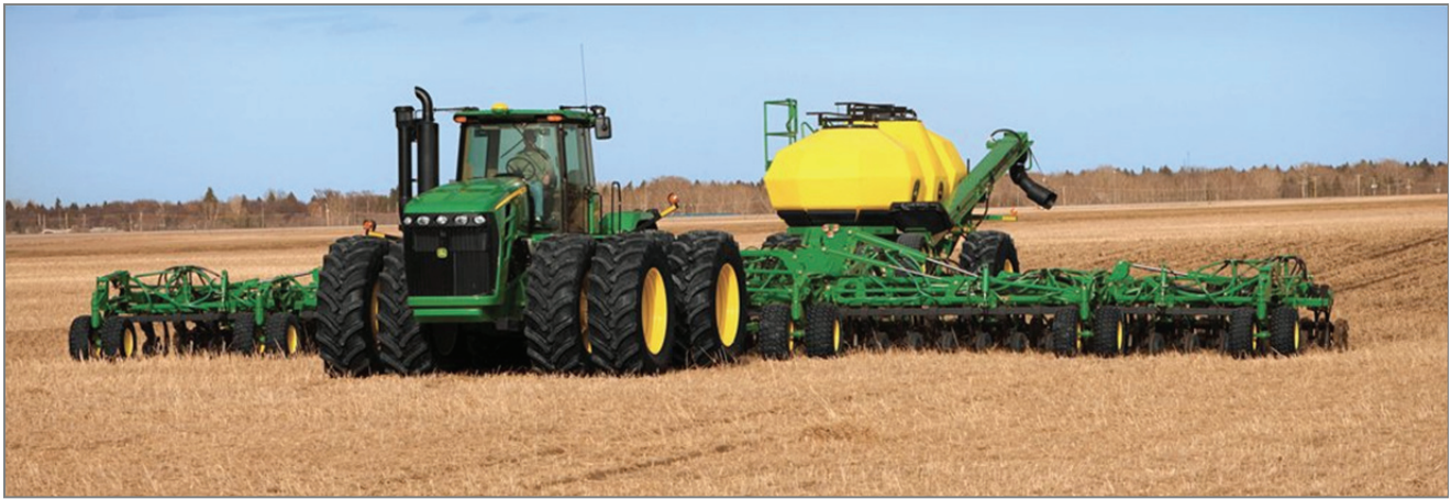
Figure 18. An air seeder, which benefits from multiple hydraulic systems.
