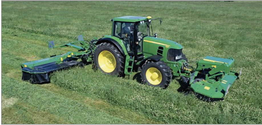
Figure 6. A front-mounted mower conditioner is a typical application requiring a front PTO and a front hitch.
