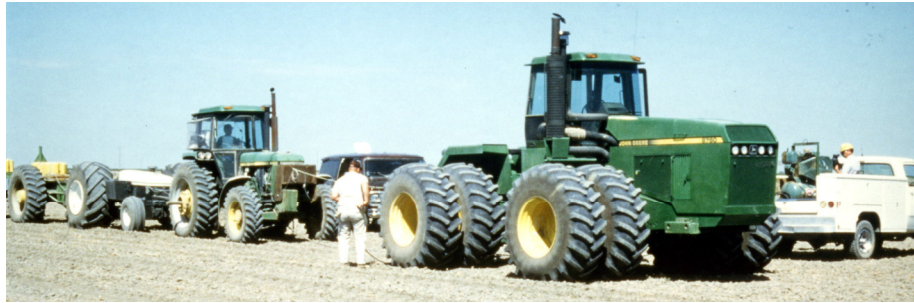
Figure 30. 4WD power hop testing in the San Joaquin Valley of California, 1990.
