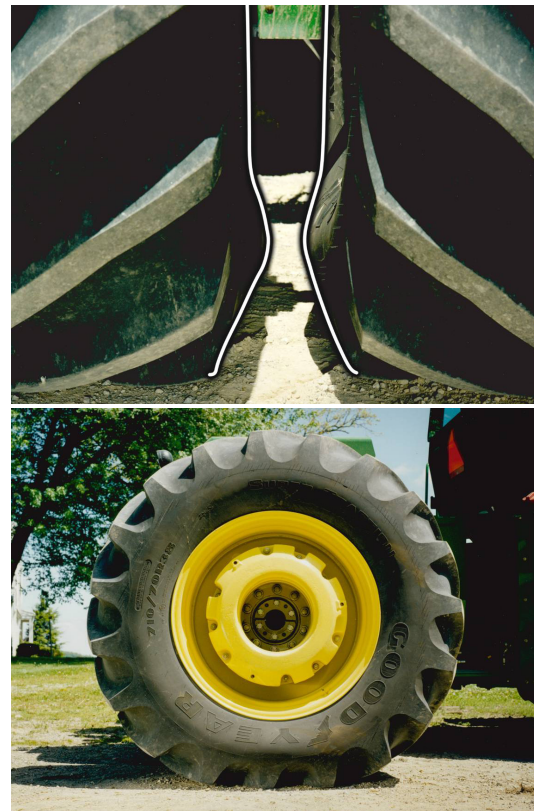
Figure 32. Radial tires inflated correctly with Rated Deflection Pressures.
