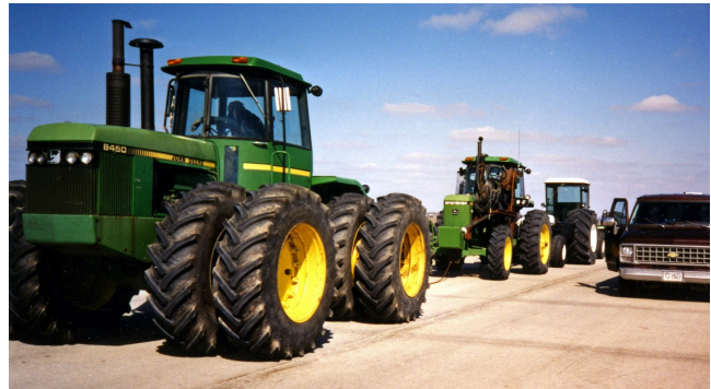
Figure 27. John Deere 8450 power hop testing on concrete in 1990.
