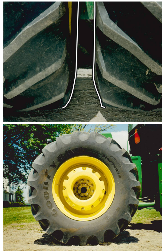
Figure 33. Overinflated radial tires.
