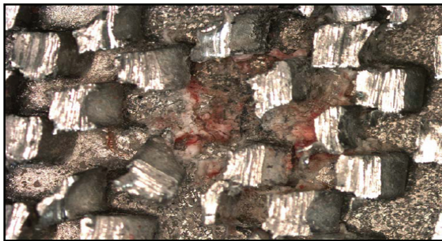
Figure 19. Internal corrosion site in an aluminum heat exchanger (magnification 10X).
