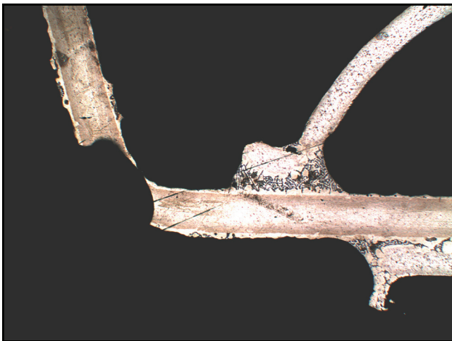
Figure 23. Cross section of the erosion pit from Figure 21.
