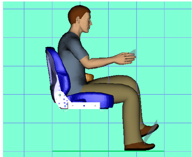
Figure 4. Human inserted to SIP showing ISO 4253 zones.
