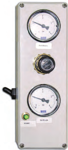
Figure 12: Analog operating panel. Source: PTG.
