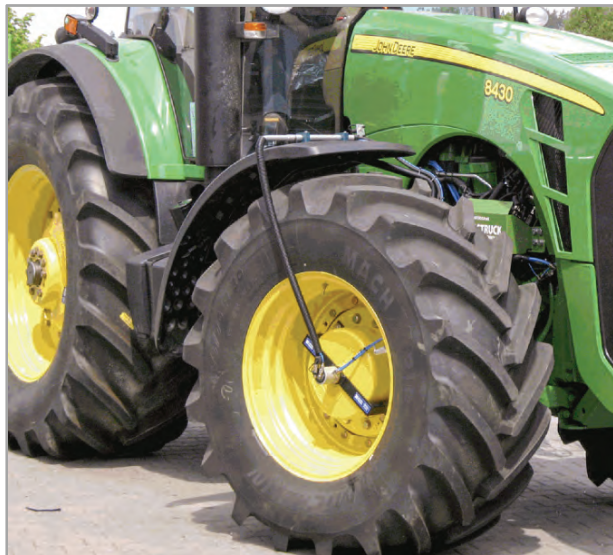
Figure 20: JD Tractor equipped with CTIS on front and rear axles. Source: PTG.
