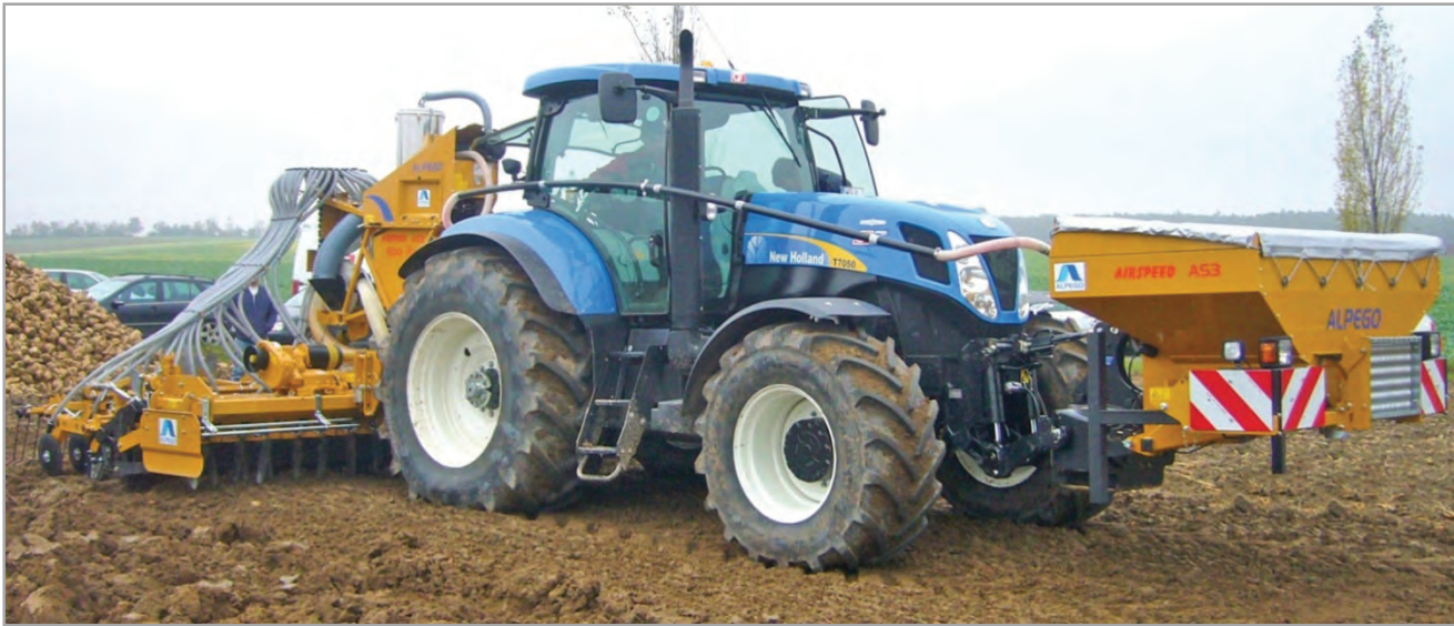
Figure 1: NH Tractor with CTIS on the rear axle. Source: PTG.
