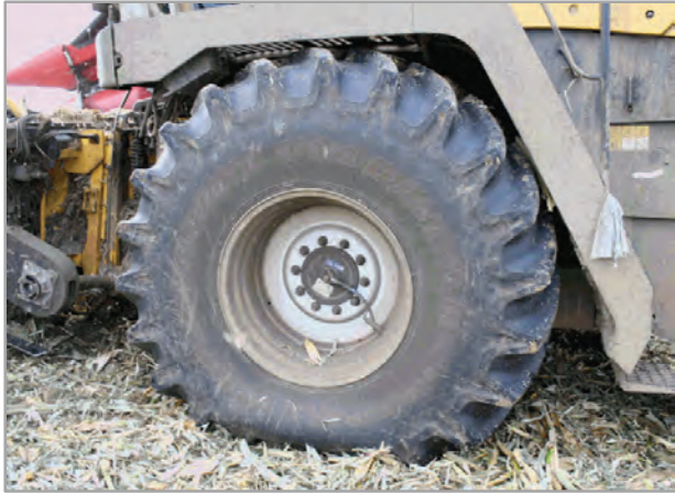
Figure 26: Self-propelled harvester equipped with CTIS on the front axle. Source: PTG.
