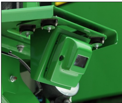
Figure 9. AutoTrac Vision front mounted camera for crop-referenced guidance (source: John Deere, www.deere.com ).
