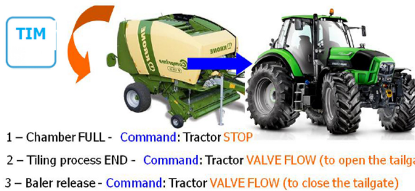
Figure 16. Commands from the implement to the tractor for a Krone baler (source: www.europeanlandowners.org ).
