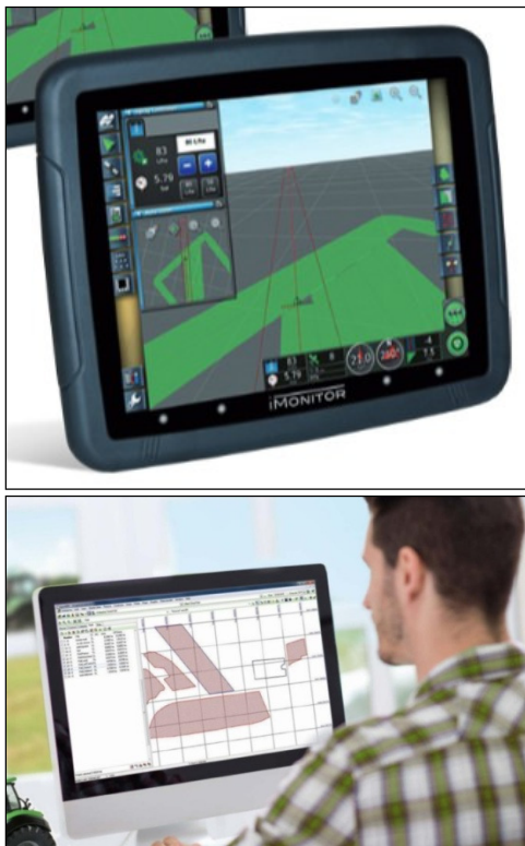
Figure 23. Job planning on iMonitor and on desktop in the office (source: AGROSKY, http://www.deutz-fahr.com/en-gb/search-results/1220-agrosky ).
