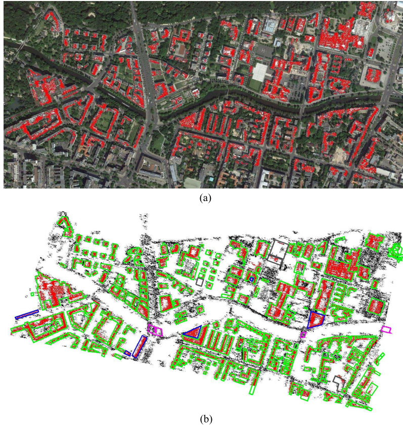
Fig. 12. Results of building extraction: Berlin. (a) Extracted roof points in red are overlaid onto the optical image (Google) of the area of interest. (b) Red and black points depict building and nonbuilding points, respectively. The overlaid green polygons are reference buildings downloaded from OSM [46]. Blue polygons are manually extracted buildings not present in OSM data. Gray polygons are newly constructed buildings that are not present in our data set, whereas magenta polygons are buildings that do not actually exist but are present in OSM data. Both gray and magenta polygons are not included in the evaluation.
