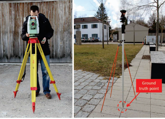
Fig. 3: (Left) Leica tachymeter. (Right) 360°prism located on top of a GTP.
