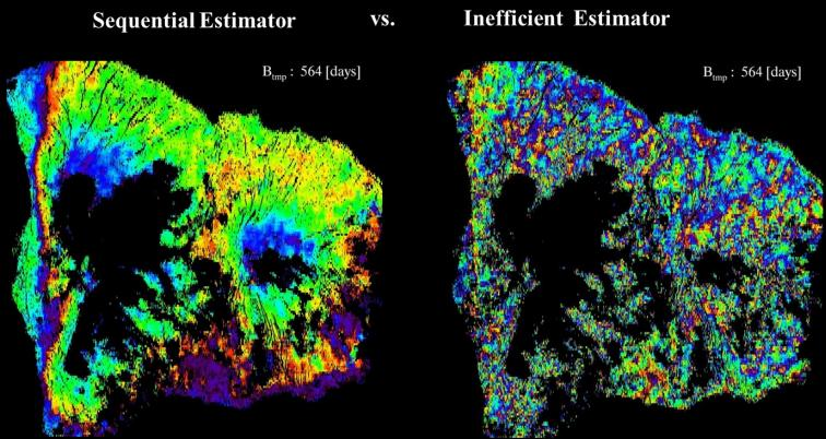
Example of the application of the proposed estimator to Time Series of Sentinel-1 Data; Salina volcanic island, Italy; Estimated interferograms with temporal baseline of 564 [days]
