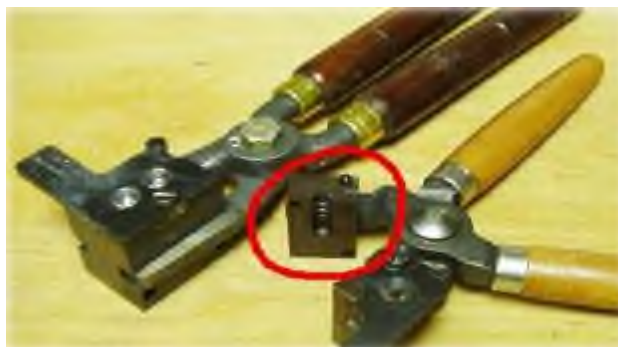
(Two bullet molds. The single cavity mold is open and empty. The double cavity mold is closed and contains two bullets. Photo Credits: Thewellman)
