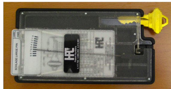
Figure 2: A manual key decoder in use. A spring loaded probe contacts the key (here at its first cut) which turns an indicator wire (here showing a depth of 6). The goal of this paper is to achieve much the same readings, but using only digital images of keys.
