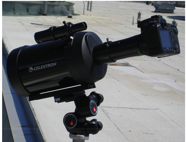
Figure 7: Telephoto setup consisting of C5 spotting scope, TeleVue PowerMate 4X Tele-extender, and Canon 40D Digital SLR. Entire system folds up into two small cases and weighs 16 pounds.
