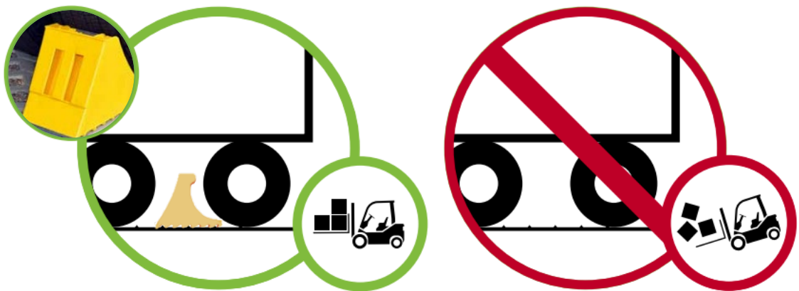
Figure 1: Example of a suitable vehicle restraint system in place (left image, green) vs. no restraint system in place (right image, red)
