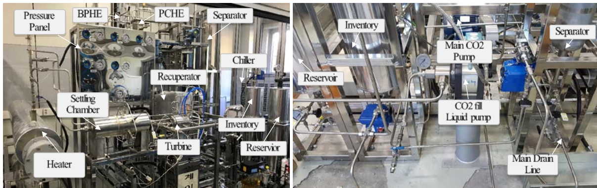
Figure 5: Schematic of kWe-class sCO 2 transcritical cycle test loop [8]
