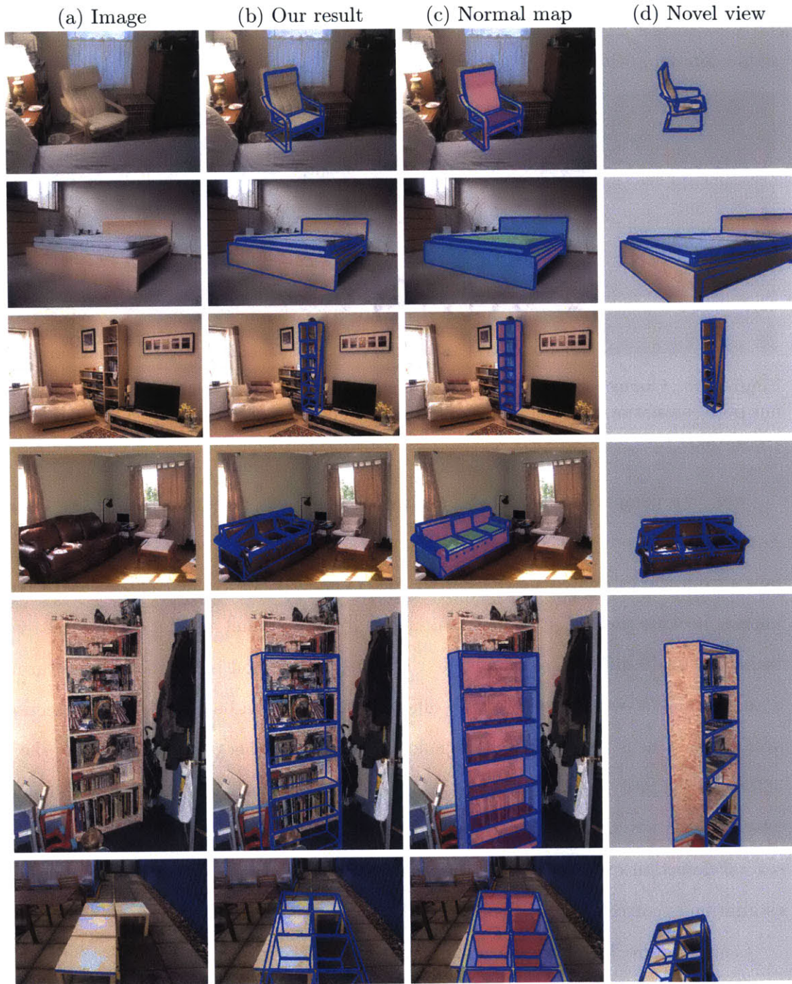
Figure 2.9: Final results: we show qualitative results of our method. (b) shows our estimated pose, (c) shows a normal direction, and (d) shows a synthesized novel view by rotating along y -axis. First 4 rows are correct estimations and last 2 rows are incorrect. Note that an error on the 5th row is misaligning a bookcase by 1 shelf. Near symmetry and repetition cause this type of top false positives.
