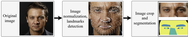
Fig. 7. Preprocessing of a sample from the CelebAMask-HQ dataset: face and face landmarks are detected for image normalization and eyes’ region image crop and segmentation.
