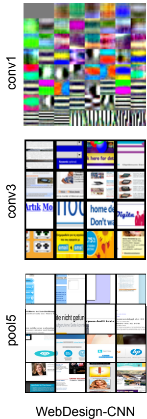
Figure 7: Visualization of WebDesign-CNN neurons at different layers. We show all 64 filters for conv1 units and four sample filters for conv3 and pool5. Noticeably, the WebDesign-CNN learns mostly horizontal and vertical edges (conv1), simple shapes (conv3), and more complex visual patterns like logos and faces (pool5).
