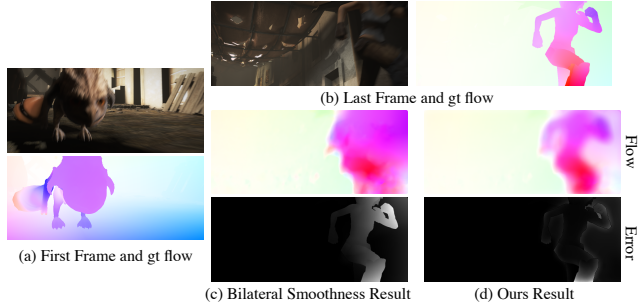
Figure 8: (a) the first frame and its GT flow from a training sequence from the Sintel flow dataset; (b) the last frame and its GT flow from the same sequence; (c) flow estimate with bilateral regularization and its error map; (d) flow estimate with our and its error map. Error maps are scaled between 0 (black) and 5 (white).
