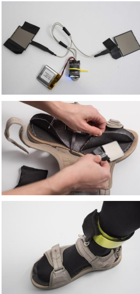
Figure 2: Overview of the wearable prototype, which includes force-sensitive resistors (FSRs) in the shoe insoles and a 9-axis movement sensor (IMU) worn on the lower leg. Note that the device can be easily modified to fit/sonify another part of the body (e.g. upper leg, arm, trunk).
